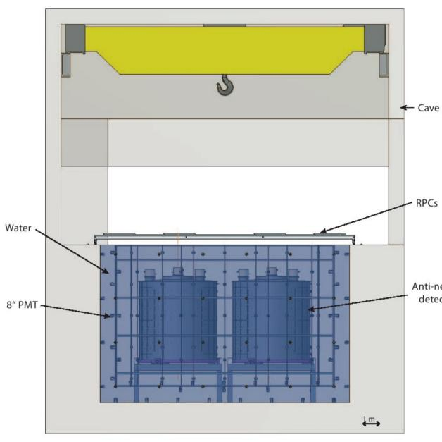
a 2.5 m active water shield around the antineutrino detectors instrumented with 8-inch PMTs
